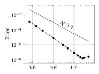
Fig. 4. The solution error compared to the theoretical estimate  $N^{-3/2}$  with  $\epsilon = 10^{-6}$
