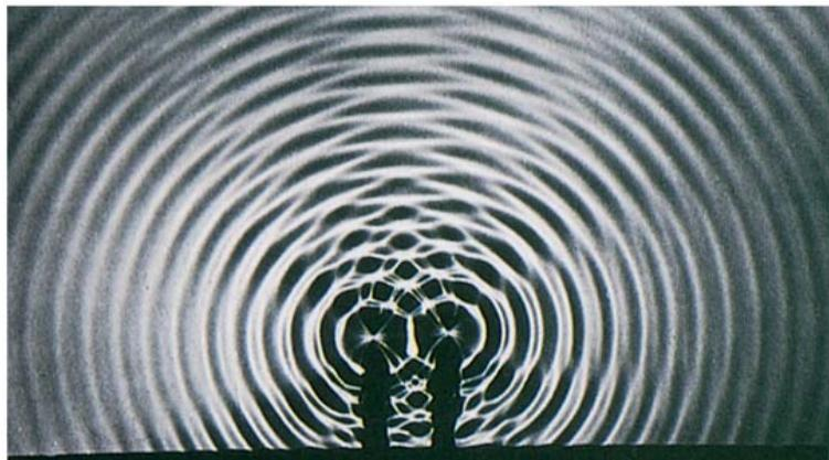
$$A_{\text{res}} = 2A \cos\left(\frac{1}{2}\delta\right) \quad \text{und} \quad \delta = 2\pi \frac{\Delta r}{\lambda}$$
