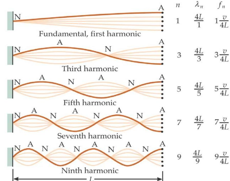
Again, an easy way to remember the resonance frequencies given by Equation 16-13 is to sketch Figure 16-16 to remind yourself of the standing-wave condition and use  $v = f_n \lambda_n$
