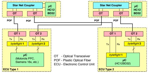
Figure 7 - Redundancy concept
