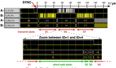
Figure 2 - Distributed synchronized slot counters
