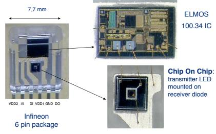
Figure 5 - Optical transceiver for bidirectional transmission
