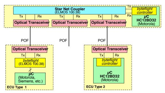
Figure 6 - Example of a byteflight topology
