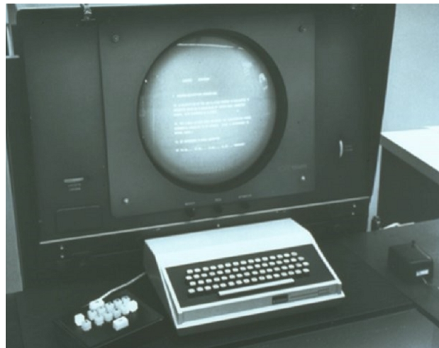
figure 3. Showing the raster scan video screen and keyboard in the middle, the chord-keyboard left and the mouse right.
