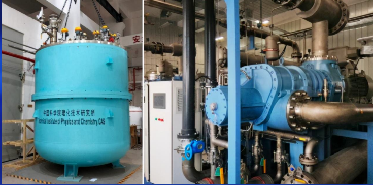
-271°C Superfluid Helium Large-scale Cryogenic Refrigeration Equipment (2021)
